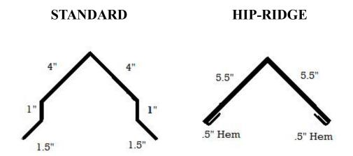
The Ridge Cap is used to seal the point at which two upward slopes meet. This can be both along the ridge of the roof as well as a covering for a hip. Self-drilling lap TEK screws are applied through the Ridge Cap into the ribs of the metal roofing panels. Debris, insects, or prevailing rain can find easy access under the ridge cap, so closures are often used to either totally or partially seal the opening. Closures under ridge caps are available in 3 types: solid, vented, and universal type.
