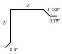
Gable flashing is used to trim the edge of the roofing panel at the gable end of the roof. It is made to match the eave drip in size to maintain a uniform appearance. Gable trim is necessary on most roofs to prevent rain water from getting underneath the metal panels. While not recommended, if the panel is allowed to hang over the gable end, eave drip can be used as an alternative. Butyl tape between the Gable trim and panel eliminates potential leaks.
